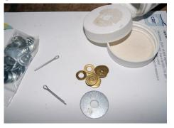
This is not precision mechanics at all: to keep the rotating arm tight and with almost no play, I needed a set of washers of different sizes both under and above the aluminium strip. At the end, instead of a cotter pin, I used a nail for the horizontal arm. Obviously, the washers' internal diameter has to be slightly above the diameter of the shaft, with as little tolerance as possible.
