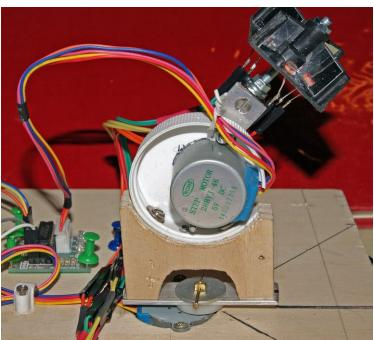
The "sensor head" bearing the 4 photoresistors was obtained **from a plastic furniture feed pad** that happened to be internally divided in four sectors. To increase directionality, **small patches of adhesive mirror coated paper were sticked to each side of each photoresistor**.
