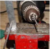
The aluminium arm needs to be kept in place on the shaft, so I very carefully **drilled a 2mm hole through the shaft**, to pass a cotter pin that would keep the arm in place. During the drilling phase, the engine was placed shaft-down, and the shaft was tightened at the edge of a small vice, so that I could drill horizontally.
